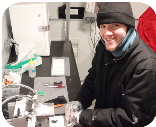
Nathan preparing an ice thin section at the National Ice Core Lab (NICL) in Denver, CO
